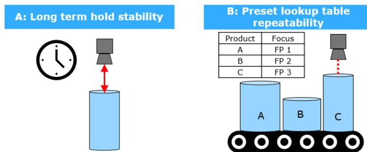
Figure 1: Illustration of the two use-cases. Case A (left) replicates a long-term hold at a unique focal power; case B (right) replicates fast re-focusing at pre-determined focal power values.
