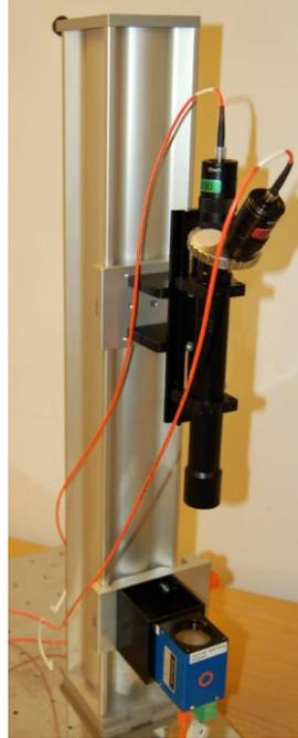
*Figure 5: Shack-Hartmann sensor with collimated light source*
